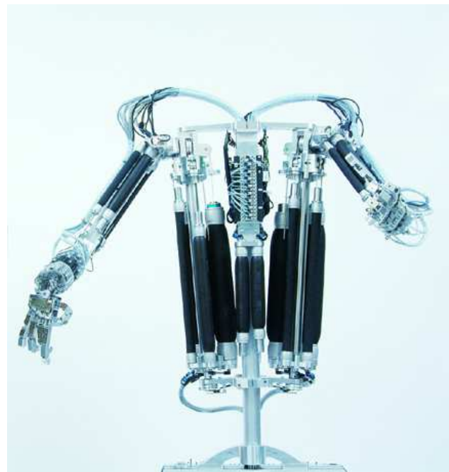
Figure 1 Photograph of the final version 5 of the humanoid muscle robot torso in action, © Festo AG & C0. KG
